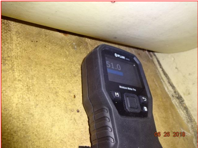
15.0 Item 2(Picture) High moisture meter reading
