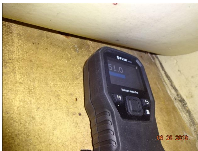
15.0 Item 2(Picture) High moisture meter reading
